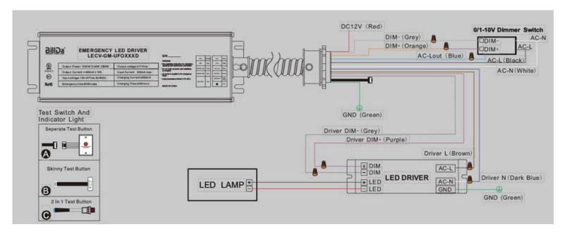
Note: This Emergency LED drivers only work with 0/1-10v dimmable LED fixture (with sensor)
